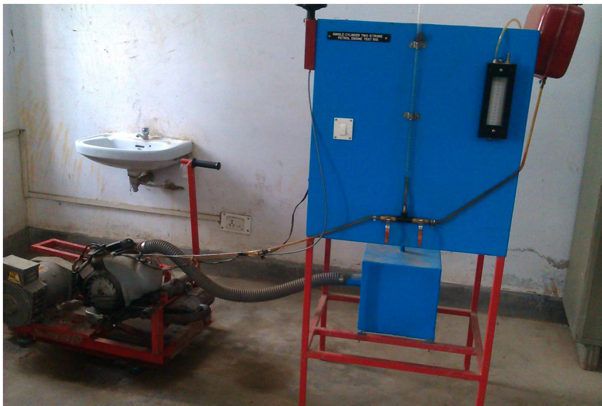
Figure.1. Experimental setup for the effect of ethanol- gasoline blends
